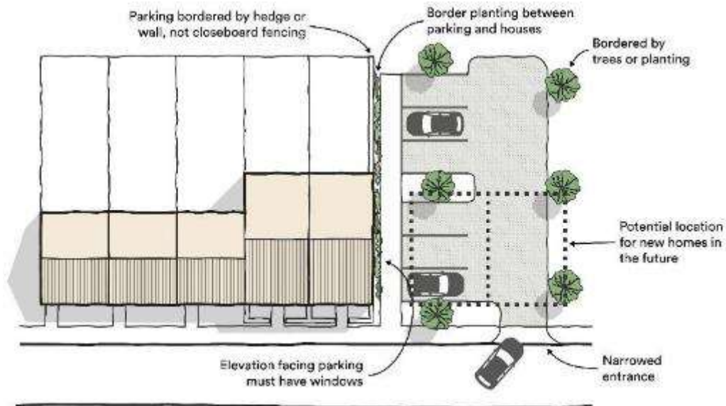
Peripheral parking forming a courtyard to the side of houses, with potential future semi-detached homes shown in a dashed line
