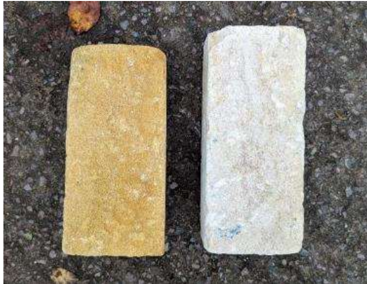
The colour of Cotswold stone in Broadway (left) is significantly yellower than the whiter variety found in the south of the Cotswolds (right)
